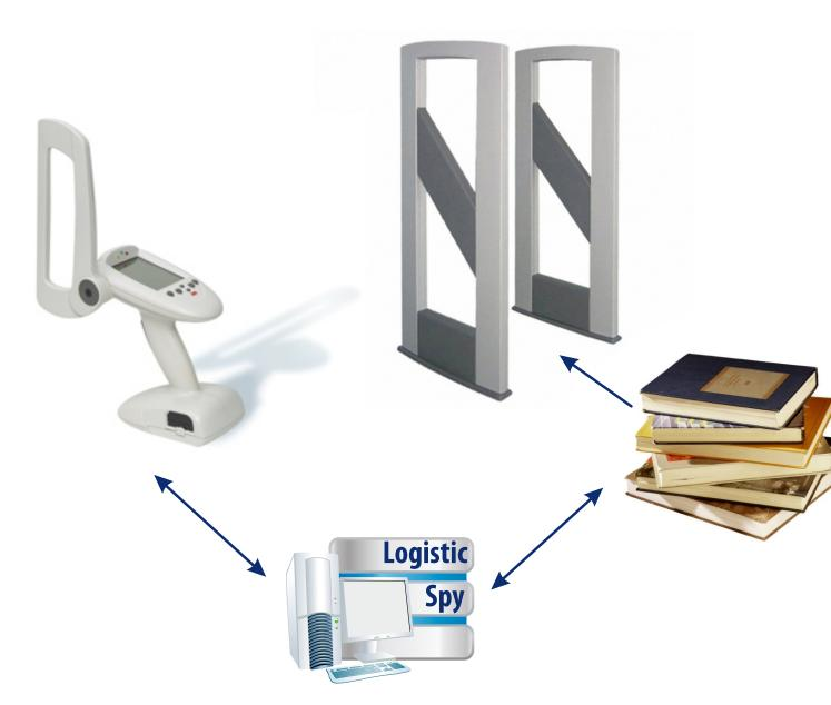
Reader accounting and library stock accounting are performed automatically by means of RFID equipment.
